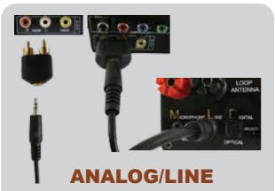
If the TV, satellite or cable box has a red and white (or black) audio output, install a 1/8" to RCA cable (not included) from this output to the "LINE" input.
